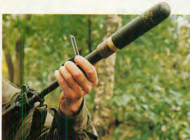
FN telescoping bullet thru rifle grenade permits the operator to launch the grenade with ball ammunition, which passes safely through the grenade. A self-sealing plug traps the propellant gases behind the bullet and uses them to launch the grenade.
